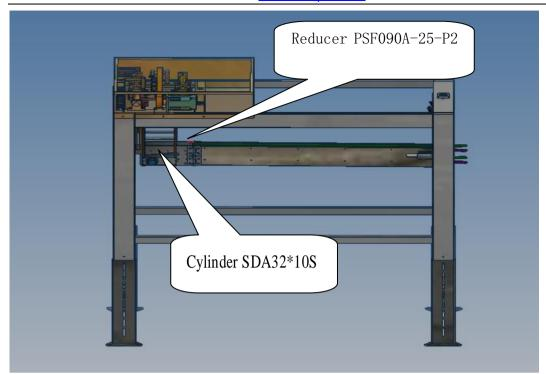
Use servo motor and synchronous belt to drive the bottle for effective and accurate left and right separation
